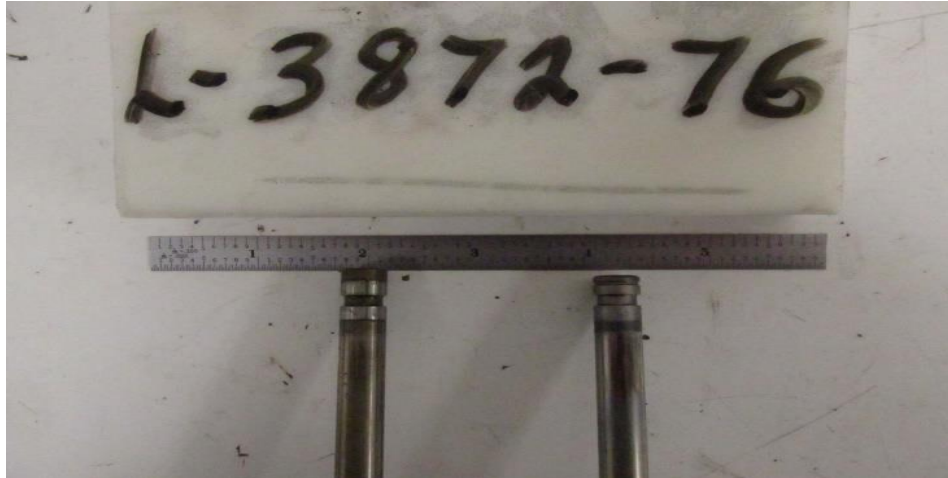
Figure 37 No. 2 Intake Valve as compared to another Intake Valve
