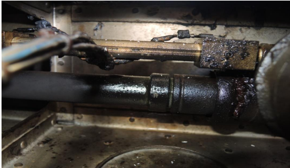
Figure 12 Wing Flap Jackscrew
