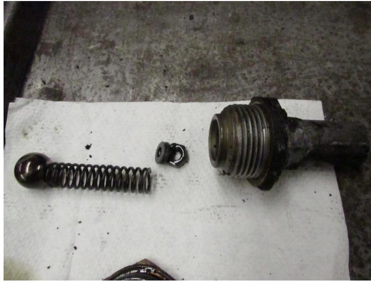
Figure 43 Oil Pressure Relief Valve
